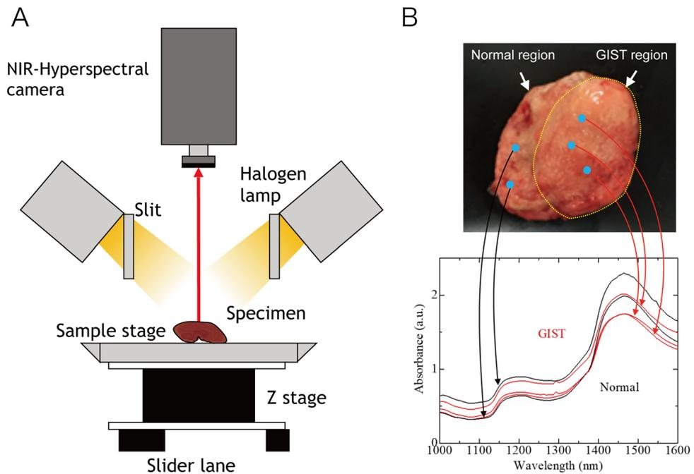
**Figure 5.** NIR-HSI system and absorbance spectra. (A) Setup of NIR-HSI system. (B) NIR absorbance spectra of HSI pixels of the GIST (Red) and normal (Black) regions. *NIR* near-infrared, *HSI* hyperspectral imaging, *GIST* gastrointestinal tumor.
